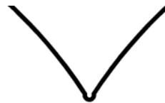
Offset is too high: bubbles appear at the corners
