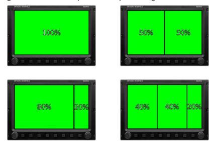
Figure 6-Example Screen Layout Configurations
