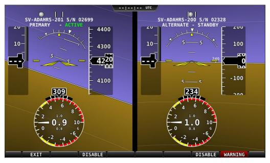
Figure 37 - ADAHRS Cross-Check Comparison
