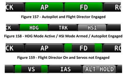
Figure 160 - VS Mode Active / ALT HOLD Mode Armed / Servos Not Engaged
