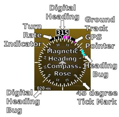
Figure 21-Example Compass Rose/Directional Gyro
