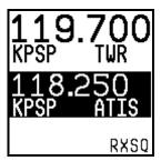
The squelch setting, which determines how strong a radio transmission must be before the radio receives it, is configured during setup. See the SkyView System Installation Guide for instructions on adjusting this parameter.
