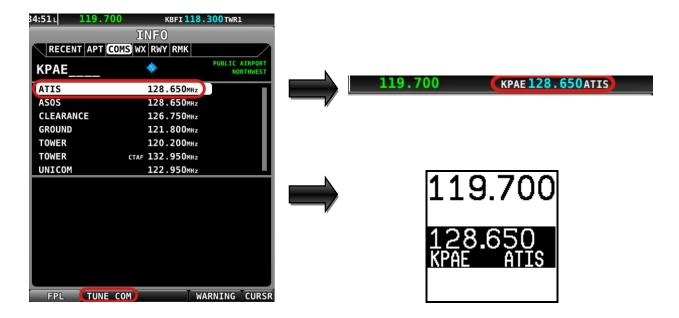
Press the dual concentric knob on the control panel to flip/flop the chosen frequency from the standby frequency to the active frequency.
