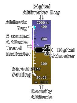
Figure 17-Example Altimeter
