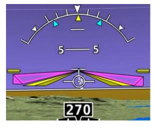
Figure 165 - Single Cue / Inverted-V with Autopilot Servos Not Engaged
