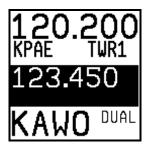
When dual watch is enabled, the SV-COM-C25 monitors the standby frequency for transmissions while simultaneously monitoring the active frequency, allowing you to listen to both (but not simultaneously). This allows you to listen to ATIS on standby, for example, while keeping tower tuned to the active frequency.
