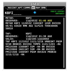
Figure 124 - METAR - Decoded
