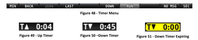
Once the TIMER menu is entered, the clock in the top bar displays TIMER information instead of the local or UTC clock that is normally shown. Leaving the timer menu will restore the clock if a timer is not running.
