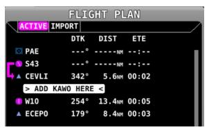
Figure 103 - Flight Plan Waypoint Insertion
