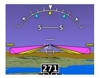
Figure 164 - Single Cue / Inverted-V with Autopilot Servos Engaged
