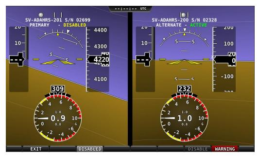
Figure 38 - ADAHRS Cross-Check Comparison (one ADAHRS disabled)
