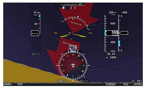
Figure 35-Extreme Pitch Warning Indicator Arrows
