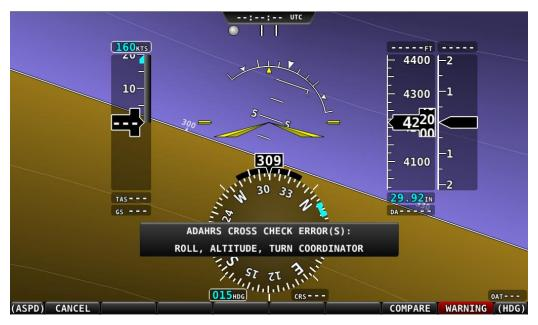
Figure 36 - ADAHRS Cross-Checking Disagreement
