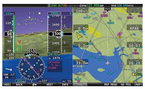
Figure 105 - Active Flight Plan: Map and Flight Plan View
