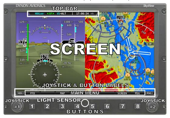
Figure 1-SkyView Display Front Bezel Layout
