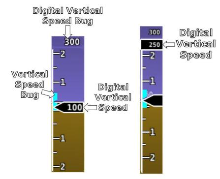
Figure 20–Example Vertical Speed Indicator.
