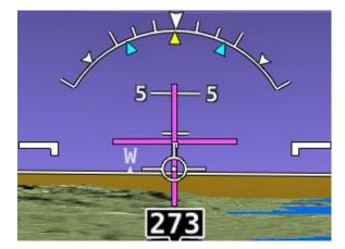
Figure 166 - Dual Cue / Cross Bars with Autopilot Servos Engaged
