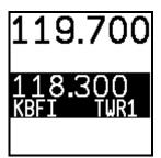
With a valid COM frequency highlighted, press the TUNE COM button to send the frequency to the standby frequency:
