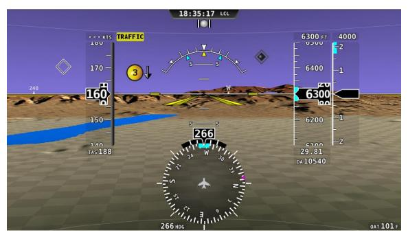
Figure 42 - Traffic Display on Synthetic Vision
