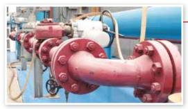
**Test Loop.** A complete Laboratory Test loop exists for design validation of WALWORTH products, performing the test at maximum design pressure and cycling the valves from 3000 to 5000 cycles. The test takes more than four months to be completed.
