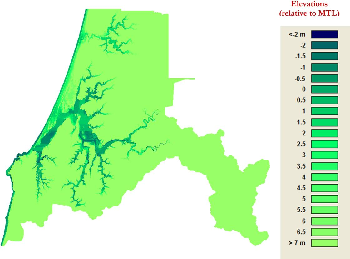
Figure 129. LiDAR elevation data for Site 8 – Coos
