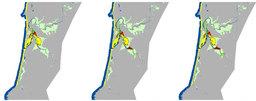
Figure 42. Wetland data for Site 3 – Nestucca. Initial condition - 2002 (left), 2100 under the A1B mean scenario (0.39 m SLR by 2100, middle), 2100 under the A1B max scenario (0.69 m SLR by 2100, right)
