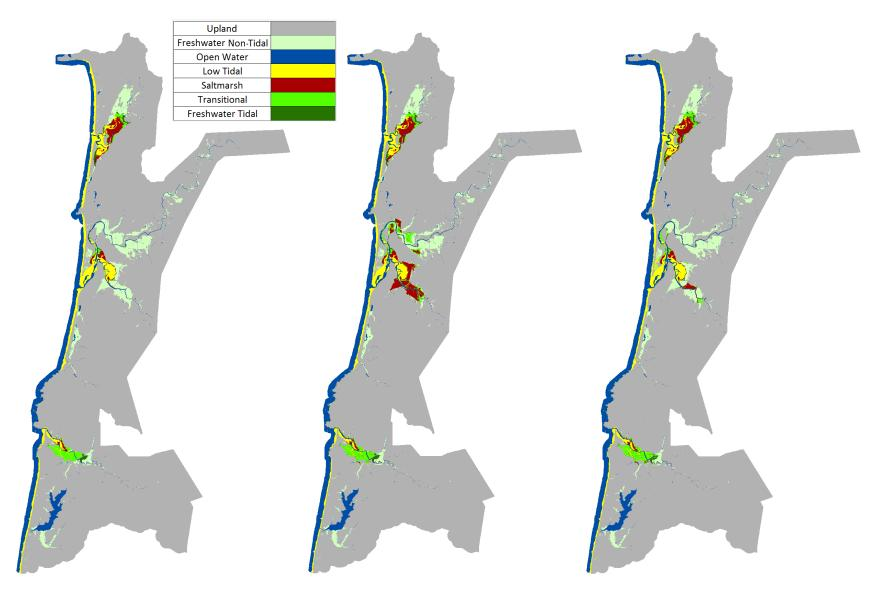
Figure 38. Wetland data for Site 3 – Nestucca. Initial condition - 2002 (left), 2100 under the A1B mean scenario (0.39 m SLR by 2100, middle), 2100 under the A1B max scenario (0.69 m SLR by 2100, right), - No Dikes
