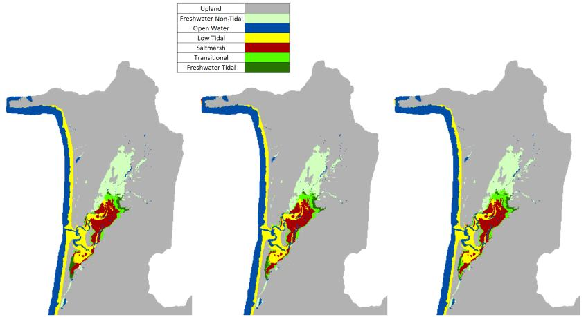
Figure 40. Wetland data for Site 3 – Sand Lake. Initial condition - 2002 (left), 2100 under the A1B mean scenario (0.39 m SLR by 2100, middle), 2100 under the A1B max scenario (0.69 m SLR by 2100, right)
