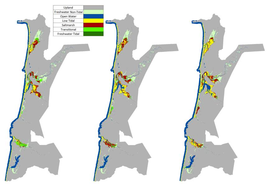
Figure 39. Projected wetland coverage in 2100 under the 1 m (left). 1.5 m (middle), and 2 m (right) SLR by 2100 scenarios - No Dikes
