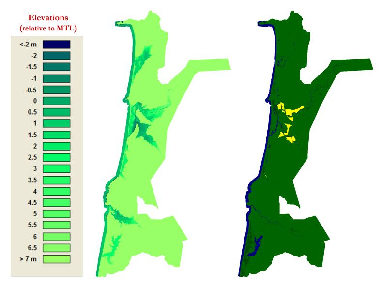
Figure 35. LiDAR elevation data (left) and location of dikes (right, shown in yellow) for Site 3 – Nestucca
