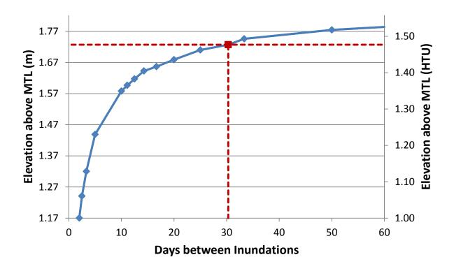
Figure 6. Inundation analysis at Garibaldi, OR
