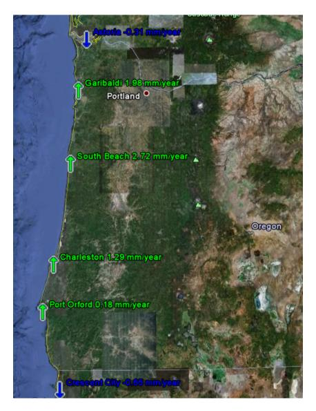
Figure 4. Locations of SLR gauge stations and observed trends on the Oregon coast
