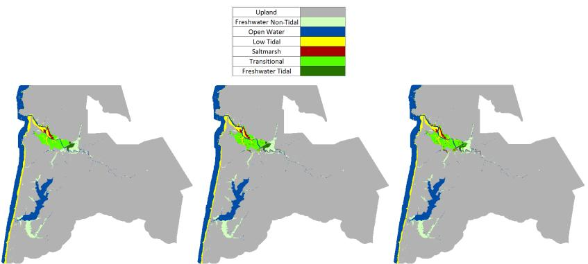
Figure 46. Wetland data for Site 3 – Salmon River. Initial condition - 2002 (left), 2100 under the A1B mean scenario (0.39 m SLR by 2100, middle), 2100 under the A1B max scenario (0.69 m SLR by 2100, right)
