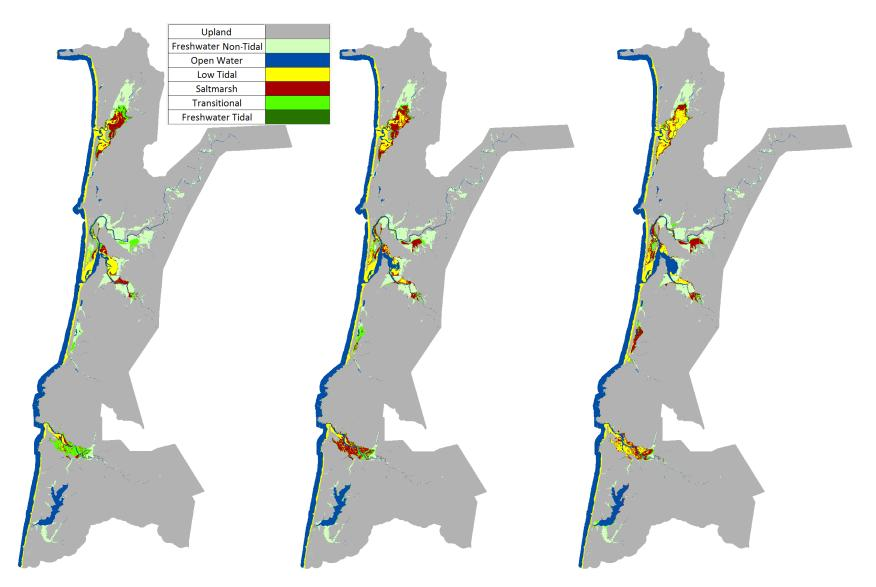
Figure 37. Projected wetland coverage in 2100 under the 1 m (left). 1.5 m (middle), and 2 m (right) SLR by 2100 scenarios
