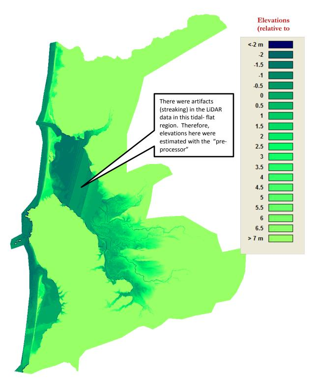
Figure 20. LiDAR and NED elevation data for Site 2 – Tillamook
