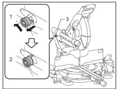
▶ 1. Unlocked position 2. Locked position 3. Stopper pin
