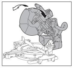
If the pointer does not indicate the  $45^{\circ}$  position, align it with  $45^{\circ}$  position by turning the adjusting bolt on the opposite side of the bevel angle scale.
