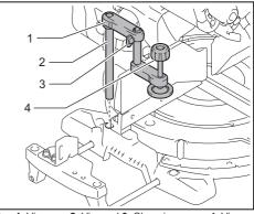
1. Vise arm 2. Vise rod 3. Clamping screw 4. Vise knob
