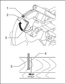
Adjusting screw 2. Range adjustment screw
