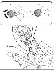
1. Unlocked position 2. Locked position 3. Stopper pin
