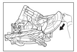
1. Remove the upper fence on the side that you are going to tilt the carriage.
