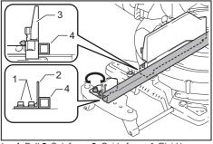
1. Bolt 2. Sub fence 3. Guide fence 4. Rigid bar
