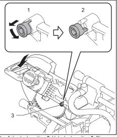
Locked position 2. Unlocked position 3. Stopper pin
