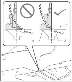
Top surface of turn base 2. Periphery of blade
