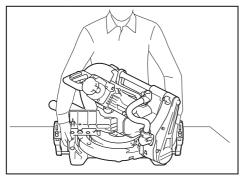
AWARNING: Stopper pin for carriage elevation is for carrying and storage purposes only and not for any cutting operations. The use of the stopper pin for cutting operations may cause unexpected movement of the saw blade resulting in kickback and serious personal injury.
