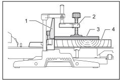
1. Upper fence 2. Vertical vise 3. Workpiece
