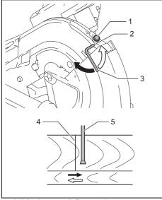
1. Adjusting screw 2. Range adjustment screw
