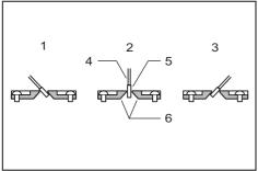
1. Left bevel cut 2. Straight cut 3. Right bevel cut
