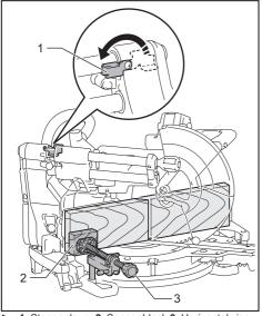
Stopper lever 2. Spacer block 3. Horizontal vise
