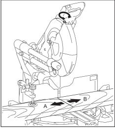
A) When you want to obtain the correct size on the left side of workpiece, shift the laser line to the left of the blade.
