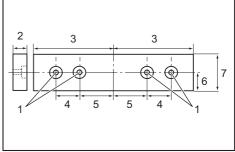
1. Hole 2. Over 15 mm 3. Over 270 mm 4. 90 mm
