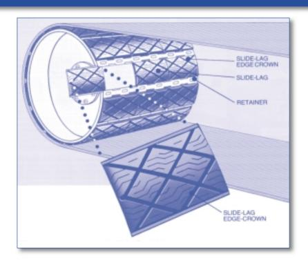
Standard conveyor engineering usually calls for a crowned surface on all drive pulleys. A crowned pulley is used to assist in tracking the belt or directing it back to the pulley center when the belt starts to wander. Eliminating erratic lateral belt movement is important in preventing damage to the belt caused by contact with the structure.
