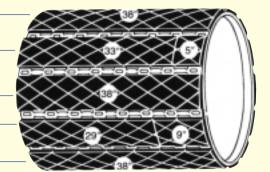
Edge-Crown® sets also make use of the butt seam application method for the pads inserted between the Edge-Crown® pads in each row; however, center sections can be provided without seams on request (Pages 5 and 8).
