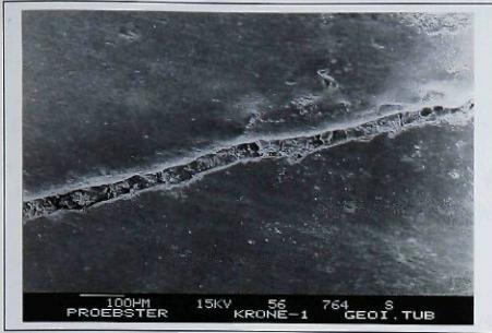
Fig 15 Marginal area of a cemented In-Ceram crown on a natural tooth. The marginal opening is in the range of 20 to 40 \mu m.
