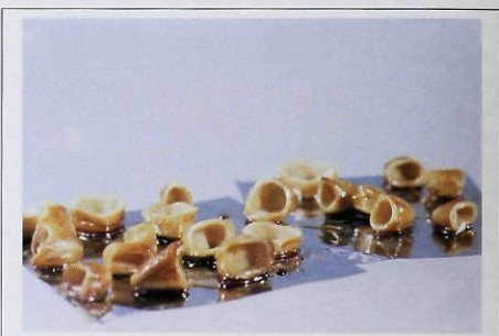
Fig 7b During firing, the frameworks soak up molten glass. Every restoration lies in excess glass.
