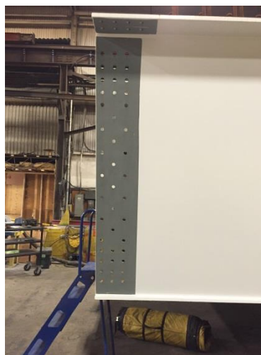
Figure 1: Masked off faying surface in shop
