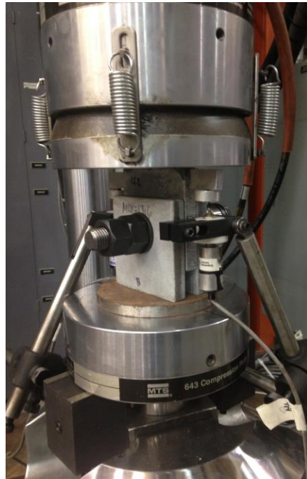
Figure 2: Short-term slip test
