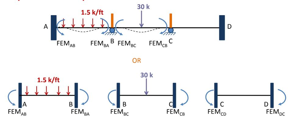
The fixed-end moments that develop at the ends of the members of this fully restrained or kinematically determinate structure can easily be evaluated by using the fixed-end moment expressions given inside the back cover of book.
