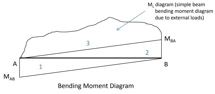
Assuming that the member is prismatic (EI is constant along the length of the member) we sum the moments of the area under the M/EI diagram about the ends B and A, respectively, to determine the tangential deviations.
