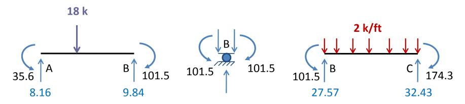
The reactions at the fixed support A and C are equal to the forces and moments at the ends of the members connected to these joints. To determine the reaction at roller support B, consider the equilibrium of the free body of joint B in the vertical direction.
