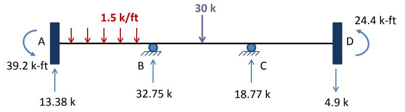
The reactions at the fixed support D equal the shear and moment at end D of the member CD.
