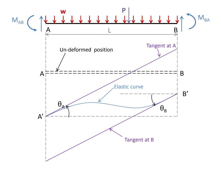
$\theta_A & \theta_B$  denote, respectively, the rotations of end A and B with respect to the un-deformed (horizontal) position of the member.
