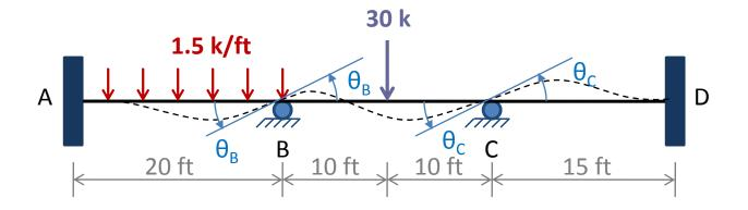
The fixed joints A and D cannot rotate, whereas joints B and C are free to rotate.
