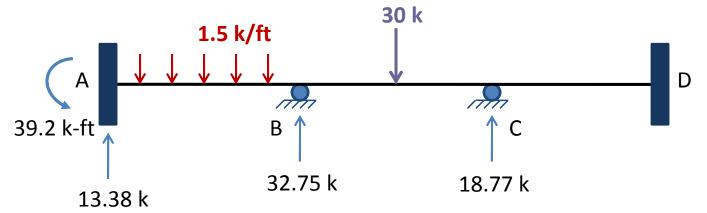
The reactions at the fixed support A are equal to the shear and moment at the end A of member AB.
