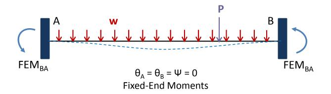
• The moments that would develop at the ends of such a fixed beam are referred to as fixed-end moments and their expression can be obtained by setting  $\theta_A = \theta_B = \Psi = 0$ ; that is,
