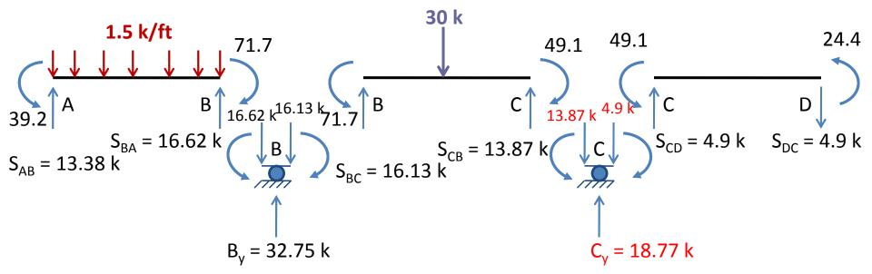
The vertical reaction at the roller support C equals the sum of shears at ends C of members BC and CD.
