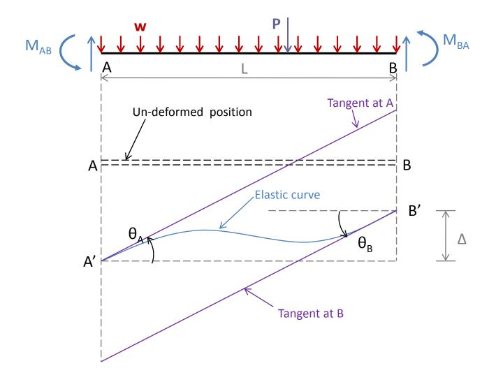
denotes the relative translation between the two ends of the member in the direction perpendicular to the un-deformed axis of the member.
