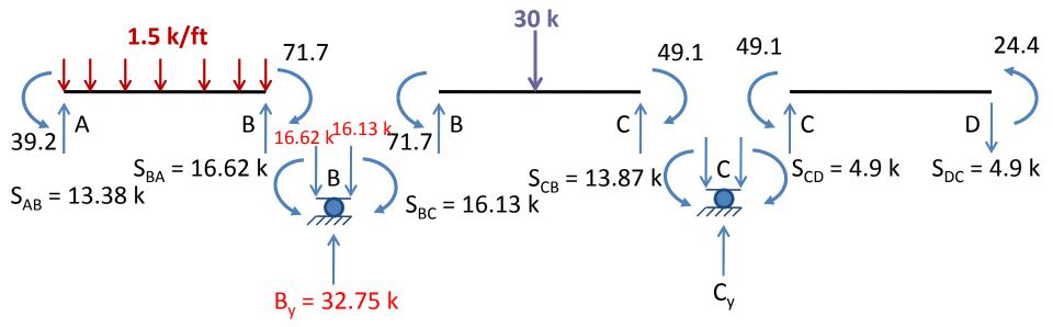
From the free body diagram of joint B, we can see that the vertical reaction at the roller support B is equal to the sum of the shears at ends B of member AB and BC; that is
