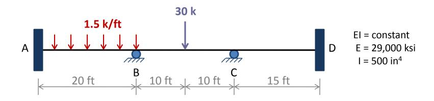
Although the structure actually consists of a single continuous beam between the fixed supports A and D, for the purpose of analysis it is considered to be composed of three members, AB, BC, and CD, rigidly connected at joints A, B, C, and D located at the supports of the structure.
