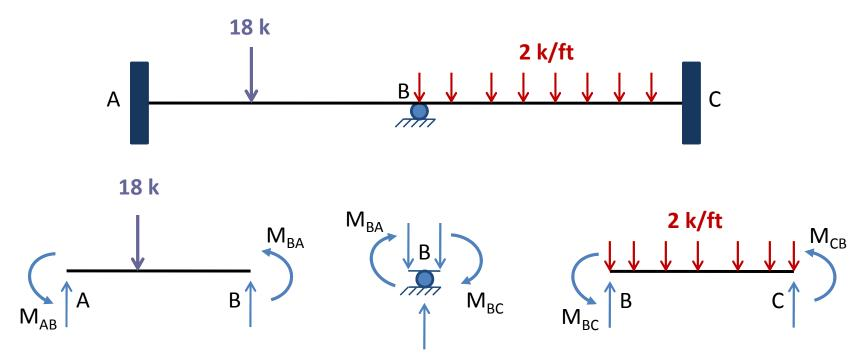
Member end moments, which are assumed to be in counterclockwise direction on the ends of members, must be applied in (opposite) clockwise direction on the free body of the joint in accordance with Newton's Third Law.
