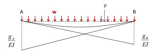
Tangential deviation due to External Loading
