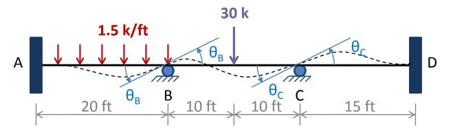
This beam has two degrees of freedom,  $\theta_B$  and  $\theta_C$ , which represent the unknown rotations of joints B and C, respectively.
