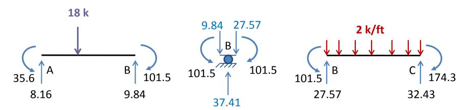
The support reactions are shown in figure below.
