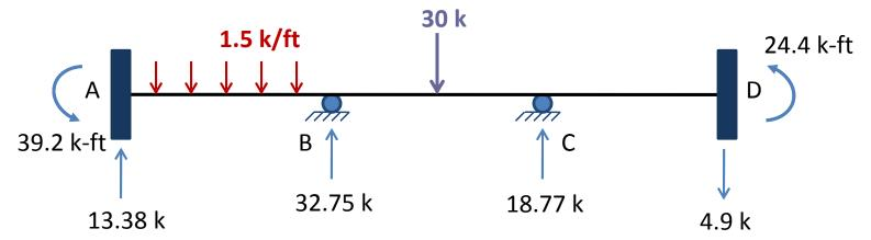
To check out computations of member end shears and support reactions, we apply the equations of equilibrium to the free body of the entire structure.
