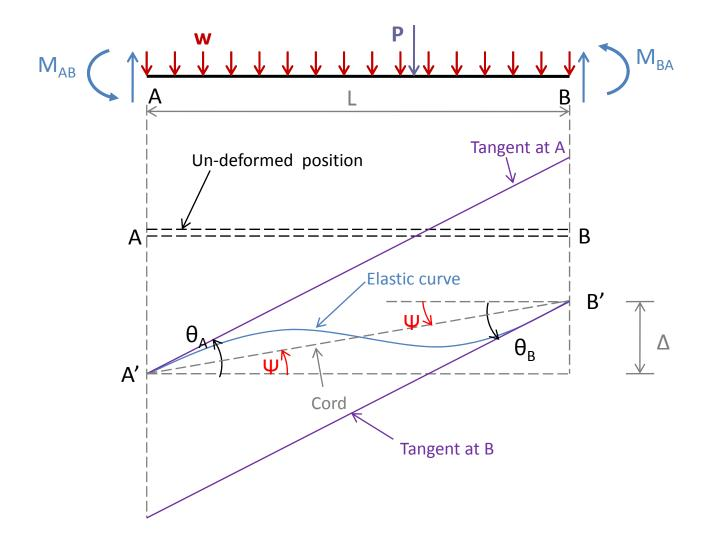
•  $\Psi$  denotes the rotation of the member's chord (straight line connecting the deformed positions of the member ends) due to the relative translation  $\Delta$ .
