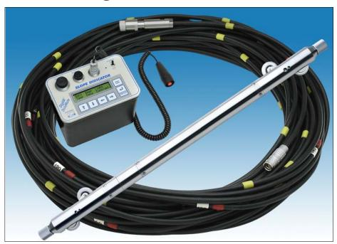
The probe is then reversed end-forend and drawn through the casing a second time. Tilt measurements from the reversed probe are used to eliminate any error due to sensor bias and to generate checksums for validating the survey.
