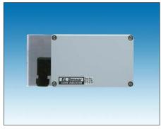
Tiltmeter with Rotating L-Bracket
