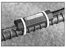
Spot-weldable strain gauge installed on reinforcing bar. The gauge is later waterproofed with mastic and
