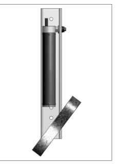
An optional embedment mounting bracket provides a way to stand tiltmeters on sloping surfaces, such as the concrete face of a rock-fill dam.
