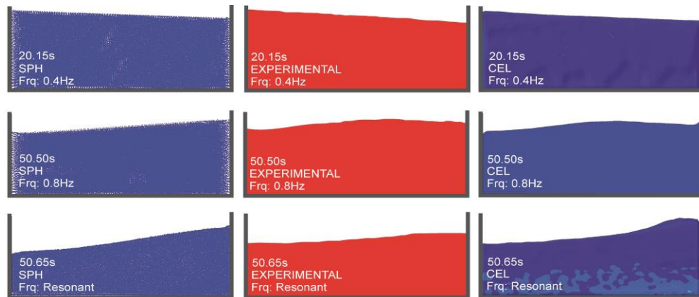
Fig.3.6. Free surface profiles of SPH, Experimental and CEL models under sinusoidal excitation with amplitude of 0.4 \text{ m.s}^{-2} at different times.
