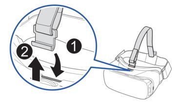
Note: The head strap contains a longer velcro strip and is used to secure the front of the Gear VR frame.
