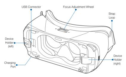
**Note**: The connected Gear VR does not require charging because it obtains power from the connected mobile device.
