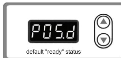
Either "**POS.d**" or "**POS.u**" will indicate "**ready**" status, depending on how the needle position is set.
