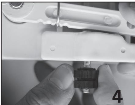
4. Turn both the screw nuts to make them move upward.
