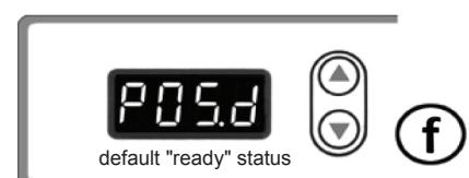
Either "POS.d" or "POS.u" will indicate "**ready**" status, depending on how the needle position is set.
