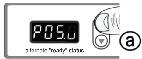
Either "POS.d" or "POS.u" will indicate **"ready" status**, depending on how the needle position is set.
