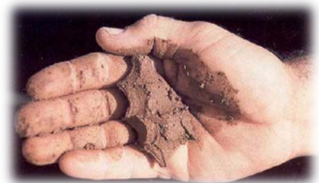
Example of estimating soil moisture by feel and appearance
