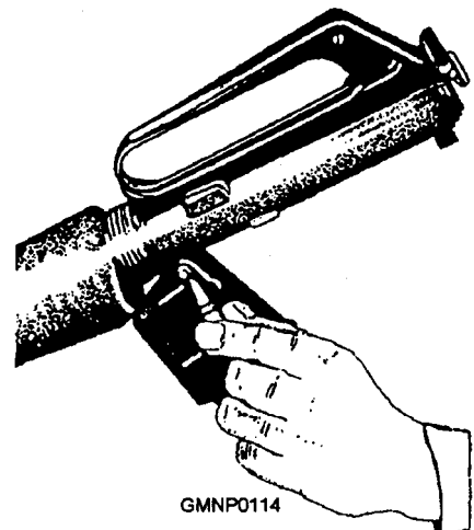
Figure 3-40.—Pressing out the receiver pivot pin.
