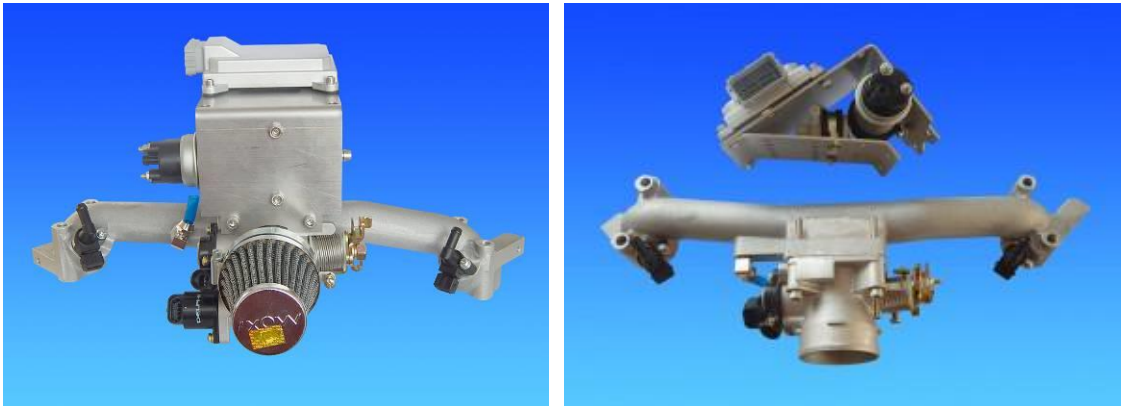
Throttle body and intake manifold assembly
