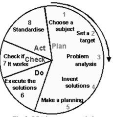
Fig. 2. SGA improvement circle Source: Own elaboration based on [9]
