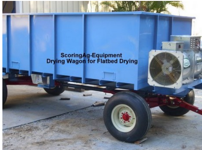
Fig: 8: Drying wagon for seeds [10]
