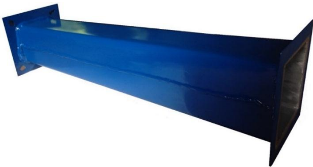
Figure 8: Small-scale wind tunnel first diffuser
