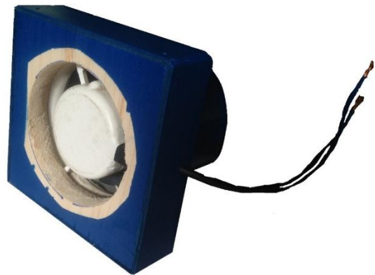
Figure 10: Small-scale wind tunnel fan
