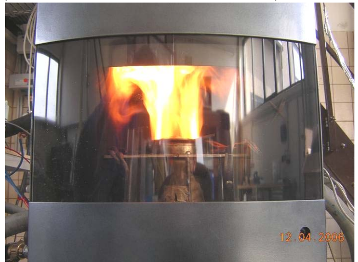
Figure 6: Combined Pellet Boiler/Stove with TEG-Prototype (located around flame in the combustion chamber)
