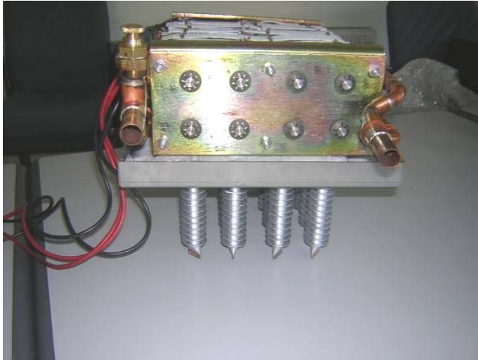
Figure 7: TEG-Prototype with Heat Pipes (bottom)
