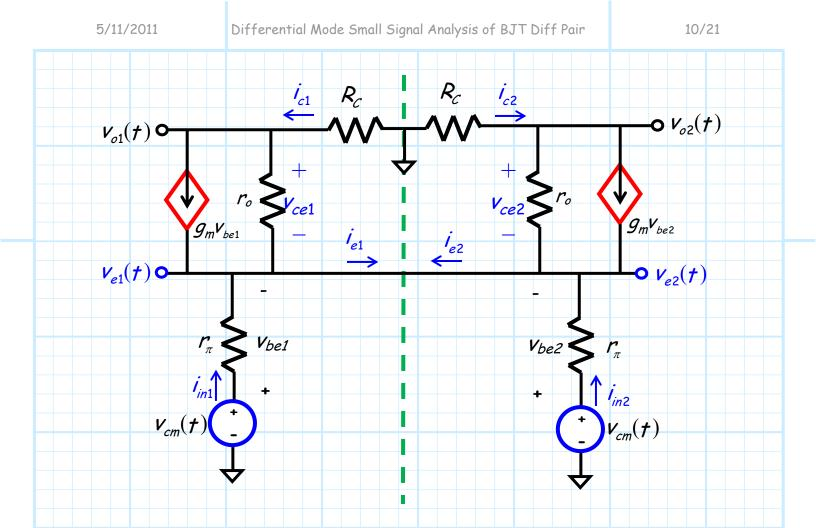
The left and right side of the circuit above are mirror images of each other (including the sources with equal value  $v_{cm}$ ).
