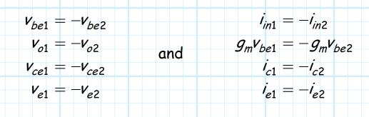
This type of circuit symmetry is referred to as **odd** symmetry: the common-mode circuit, in contrast, possessed even symmetry.
