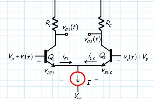
As a result, the open-circuit output voltages will likewise have a **DC** and **small-signal** component.
