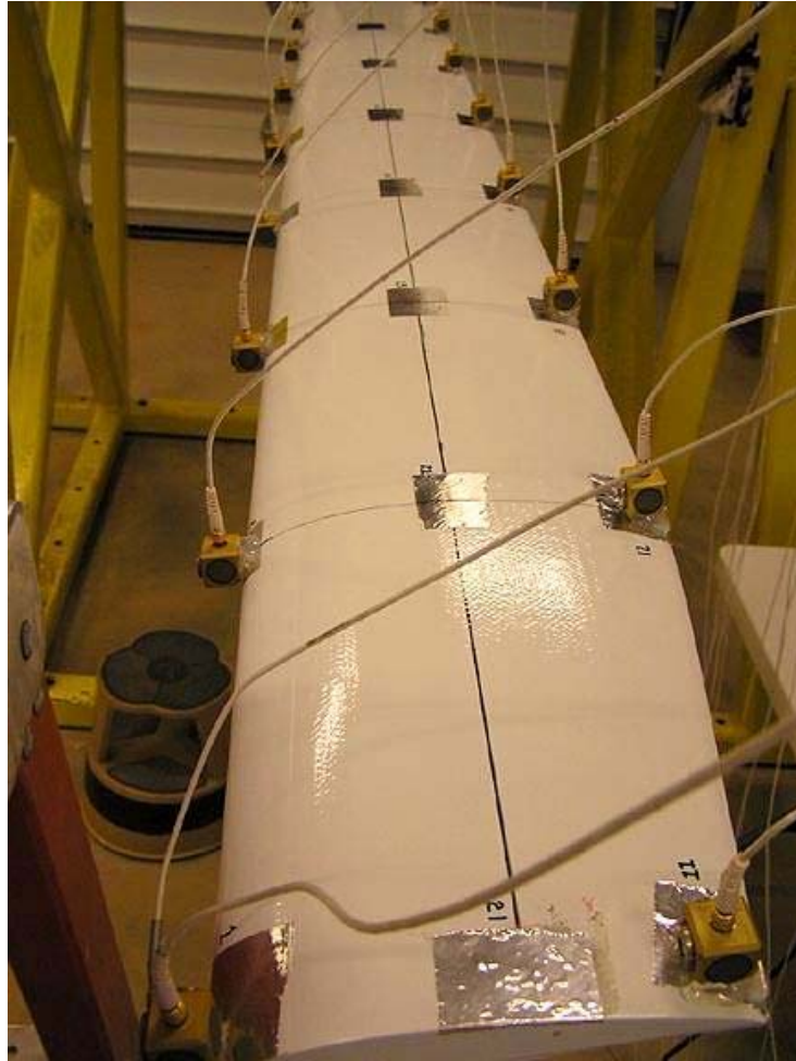
Figure B-2. Blade modal test
