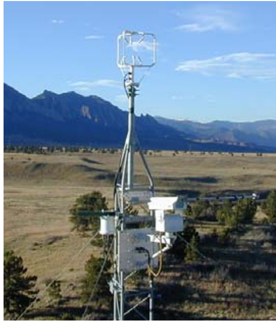
Figure 11. Sonic anemometer mounted on a meteorological tower
