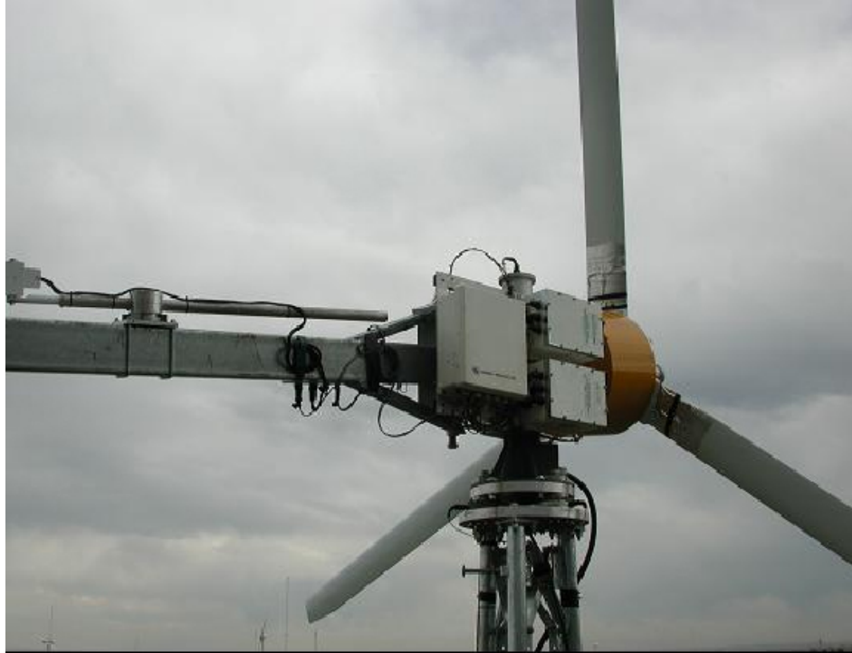
Figure 6. SWRT showing ADAS, DAMS, and Nacelle J-box
