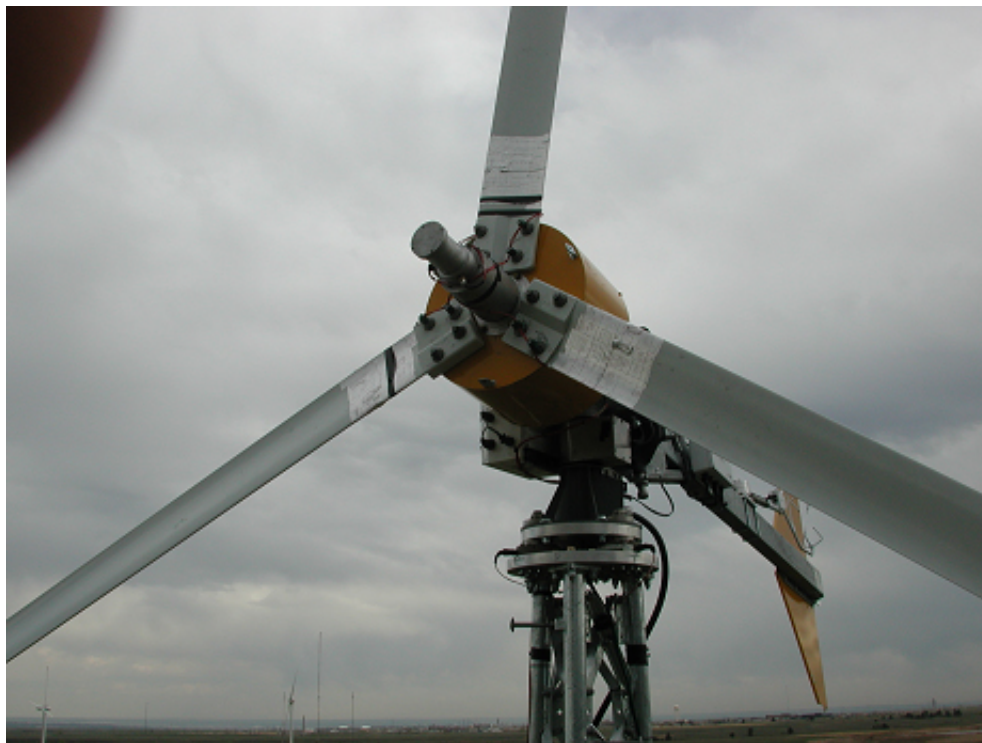
Figure 5. SWRT showing blade strain gages and rotor slip rings
