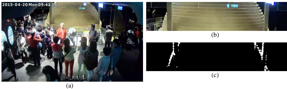
Fig. 5. (a) Screenshot from source video, (b) video cropped to tuned mass damped, and (c) pixels with valid displacements
