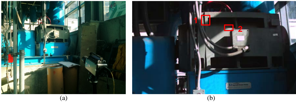
Fig. 3. Camera measurement of a motor running a pump, (a) experimental setup and (b) screenshot from video with regions of interest 1 and 2
