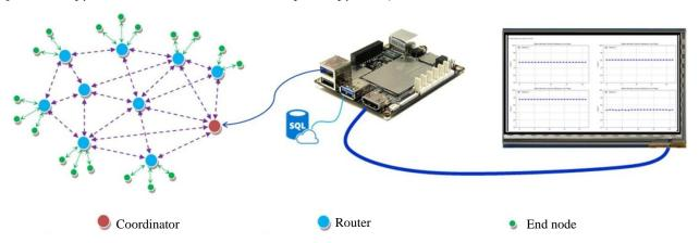
Figure 1. A typical XBee wireless sensor network system.
