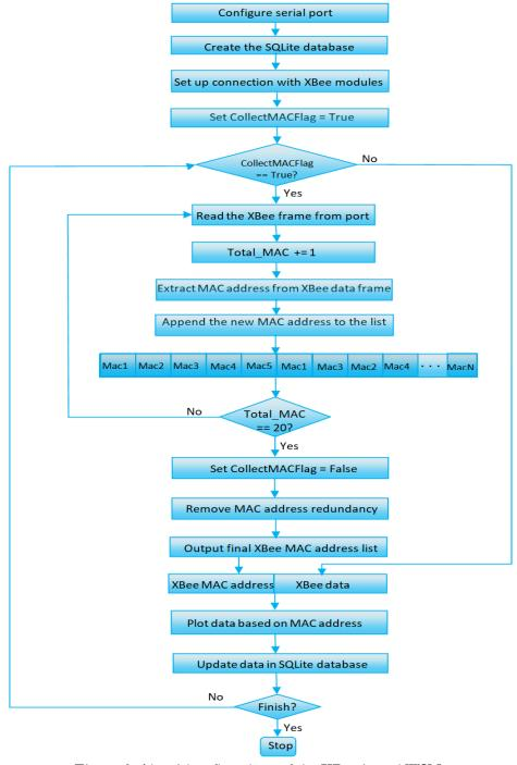
Figure 3. Algorithm flowchart of the XBee based WSN.
