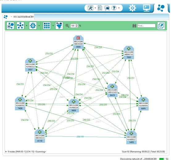
Figure 2. An XBee based WSN topology.
