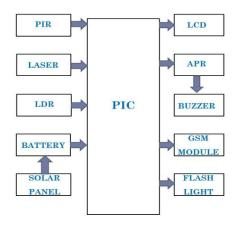
Fig.5. Block diagram of control panel.
