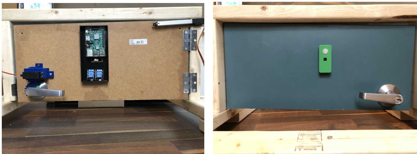
Figure 3.1 Smart Door Lock system mounted on a mockup door
