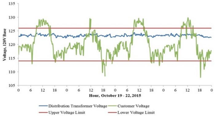
FIGURE 33. CUSTOMER-OWNED PV VOLTAGE LEVELS AT HECO
