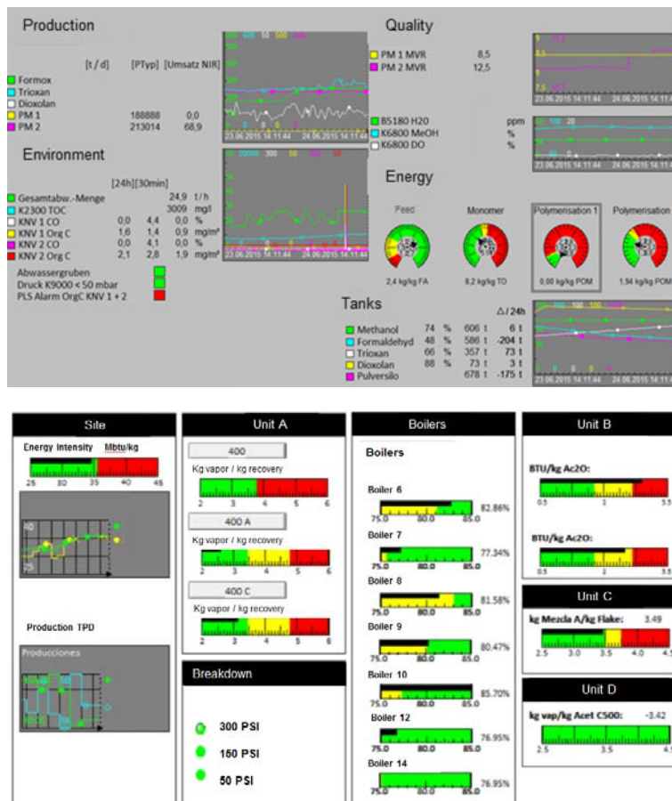
Figure 7. Energy dashboards to engage operators in energy optimization (Celanese 2016).
