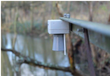
Figure 2. Photo of sea level sensor unit commercially available from https://flood.network .
