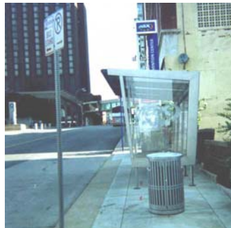
This bus shelter impedes pedestrian movement on the sidewalk.
