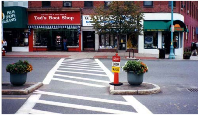
Physical islands have been demonstrated to increase the safety of pedestrian crossings. Northampton, Massachusetts supplements the island with signs advising pedestrians to pay attention to oncoming vehicles before crossing.
