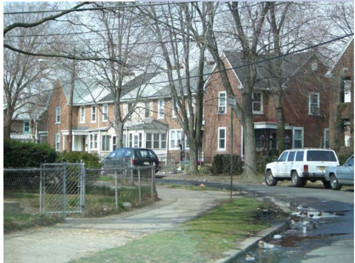
Yorkship Village in Camden, NJ. The 18 ft. roadway, on-street parking, and horizontal curves ensure that vehicles will travel slowly through this traditional planned development.
