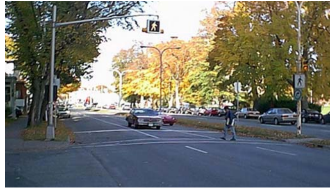
A variety of blinking pedestrian crossing signs have shown promise in increasing the yielding rate of motorists.
