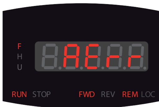
Powerfoil®X2.0 or Powerfoil®X2.0Plus Fan Keypad “Analog Error”
