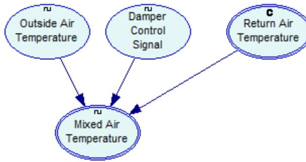
Temperature of the mixture is calculated according to the following equation:  $tma = toa * u_d + (tra - tra * u_d)$ , where  $tma$  is mixed air temperature,  $toa$  is outside air temperature,  $u_d$  is the damper signal, and  $tra$  is return air temperature.
