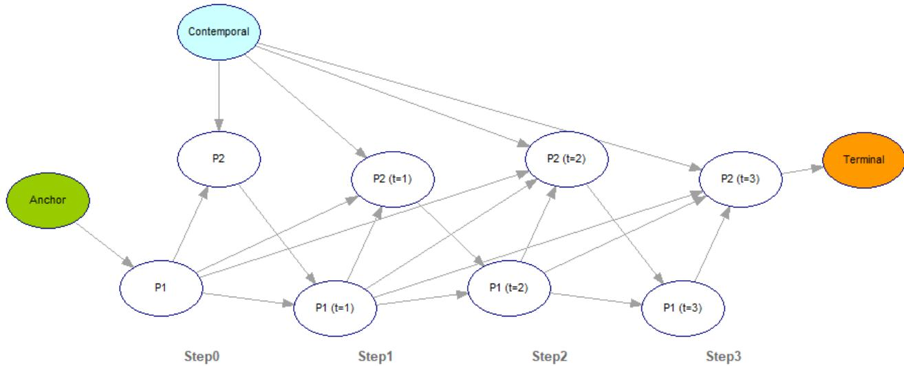
To reduce the size of the unrolled network, we changed the number of time steps (slices) from the default value of 10 to 4 with a call to `Network.setSliceCount`. The colors of the original nodes were carried over to the unrolled model, which is extended by creating new copies of the plate nodes. The structure of this network shows how the temporal arcs are used to express the conditional dependency of plate nodes in time step  $i$  on the plate nodes in time step  $j$ , where  $i > j$ .
