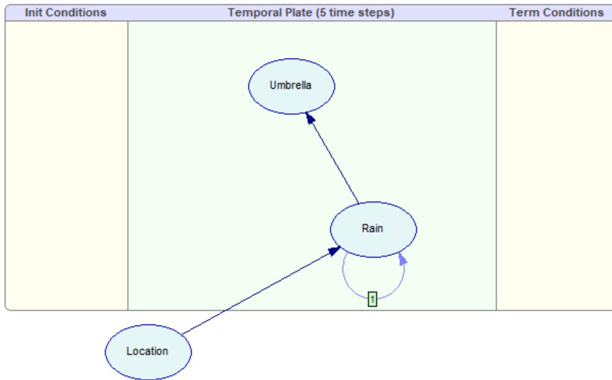
The model contains three discrete chance nodes (CPT), created with a call to `createCptNode` helper function, just like in nodes in [Tutorial 1](#)<sup>74</sup>. The *Rain* and *Umbrella* nodes are marked as belonging to the temporal plate by calling `Network.SetNodeTemporalType`:
