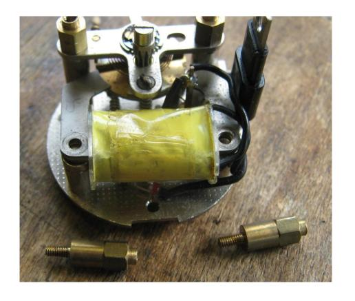
Remove 2 solenoid retaining pillars
