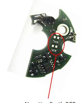
Negative Earth PCB (Resistors fitted in 2<sup>nd</sup> and 4<sup>th</sup> positions from top)
