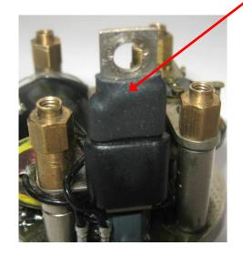
If the top of the plastic insulating sleeve is damaged, cover the damaged part with the heatshrink sleeving supplied and use a hair dryer or heat gun to shrink the sleeving over the plastic insulating sleeve
