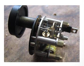
Lift off back-plate to leave mechanism as shown
