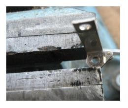
Modify connector bracket by removing side `ear' as shown
