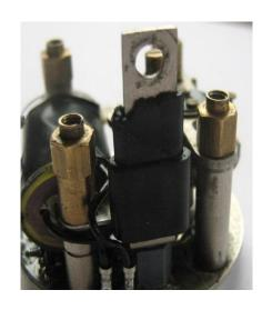
Heat-shrink sleeving shrunk over damaged insulating sleeve
