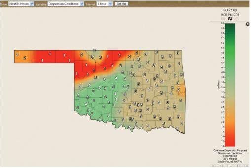
Figure 2. Example of a forecast dispersion conditions map from the Oklahoma Dispersion Model.
