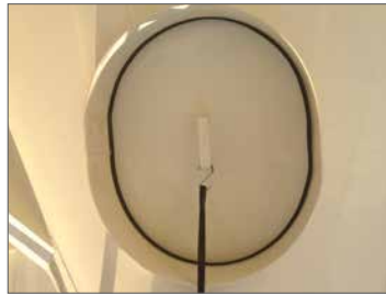
Bottom Manway Access hole in bottom cone.
