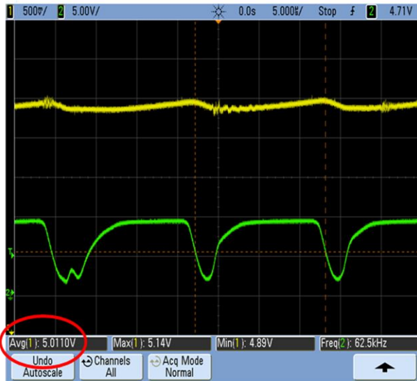
Figure 10. PWM Input to the Mosfet (Green) and Regulated Output Voltage (Yellow)
