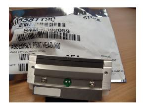
7. Place the new print head assembly onto the plastic mount bracket underneath the print station.
