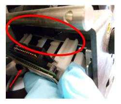
9. Reconnect the print head cable connectors, making sure that the connectors are seated tightly.
