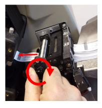
3. Using a Phillip's head screwdriver, loosen the retaining screw on the outboard end of the knife.
