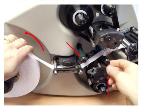
14. Rotate the **Stock Guide Knob** to center the stock.
