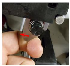
2. Press latch. Remove cores from **Upper Ink Supply Arbor** and **Upper Ink Rewind Arbor**.
