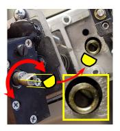
7. To insert the new knife assembly, slide it down vertically into the space between the Auxiliary Feed and the Nip Rollers.
