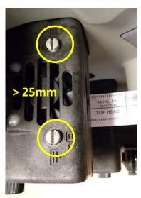
2. For stock >25mm and < 50mm, use the flat blade screwdriver to depress both buttons and turn them clockwise until they are in the lower position.
