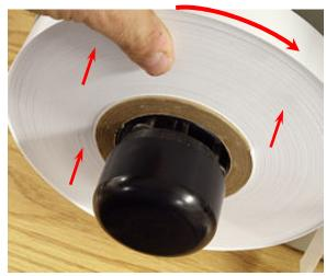
5. Rotate the **Stock Arbor Knob** clockwise quickly to extend the fingers that hold the stock.
