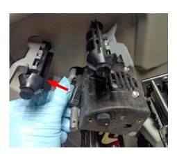
5. Press the two grey tabs on the top of the print station. Reach underneath and remove the print head from the print station.
