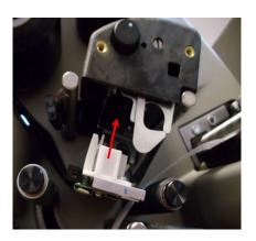
8. Carefully, align the clips into the bracket as shown. Push it up until it clicks into position.
