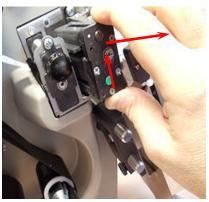
5. Clean the knife with alcohol and cotton swab. Tap the knife on a hard surface to remove cut pieces.
