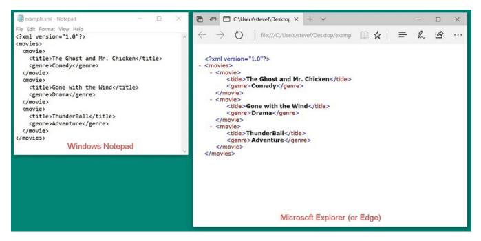
Edge and Internet Explorer automatically add DHTML code so that you can expand or collapse nodes in the tree. Internet Explorer doesn't allow you to do much besides view XML files. However, if you save your XML file with an extension of .htm or .html, IE will render the data contained in the XML file.
