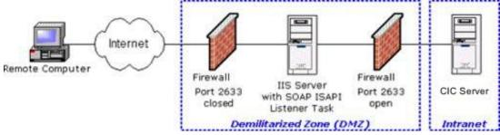
Open port 2633 on the firewall between the DMZ and the Intranet on which the CIC server is located, so that Notifier traffic can pass between the CIC server and the SOAP listener. Do not open port 2633 to the Internet.
