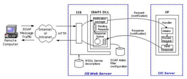
On the receiving end, the response message is decoded and used by the requesting computer in some way. This low-overhead approach permits a single server to share information with many clients.
