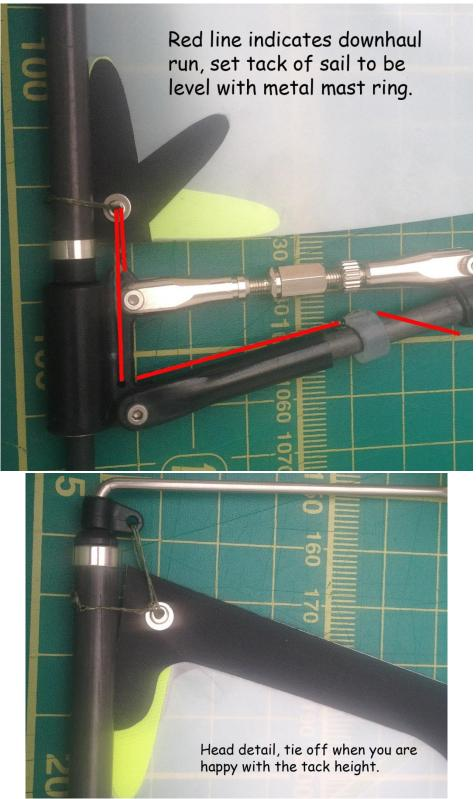
When you are happy with the height, tie off the head, then tie off the downhaul around the silicon ring.
