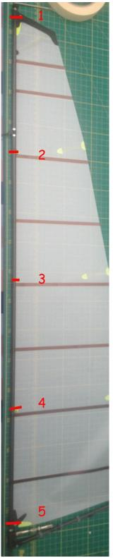
There should be a gap between the sail and the mast of around 3mm to allow the sail to rotate around the mast freely, this can be achieved by getting yourself a 3mm drill and putting it in front of the mast and tying the luff tie in place around the mast and the drill.
