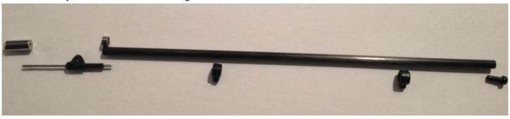
Jib Boom components, not including silicon rings
