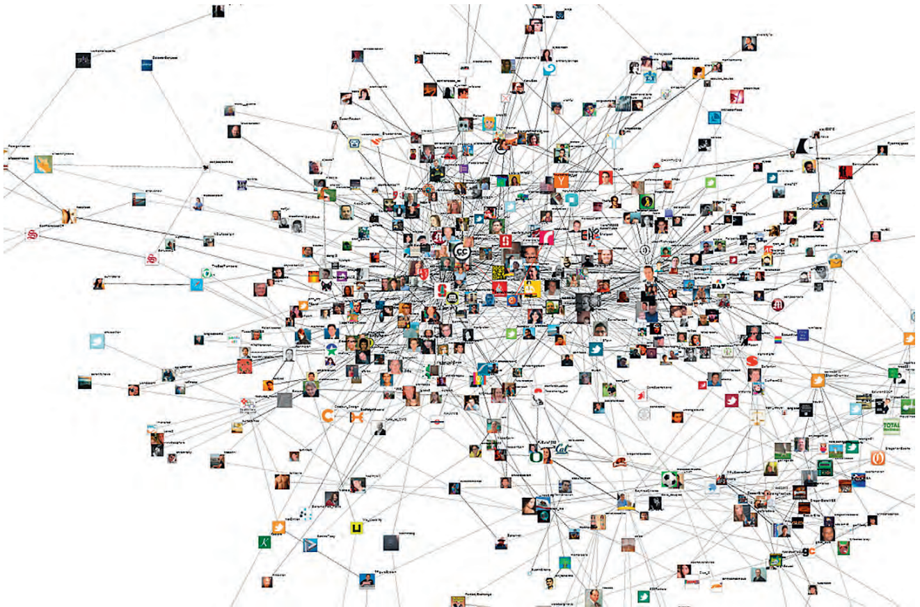
FIGURE 3.5 A medium-sized node-link network diagram visualization of Twitter users linked by patterns of following. This sized graph illustrates many issues with a network graph containing more than a few dozen vertices. Many vertices sit on or overlap with other vertices. The number of edges associated with some vertices is impossible to count, whereas other edges cannot be traced from source to destination. Improvements to network layout are an active area of research.
