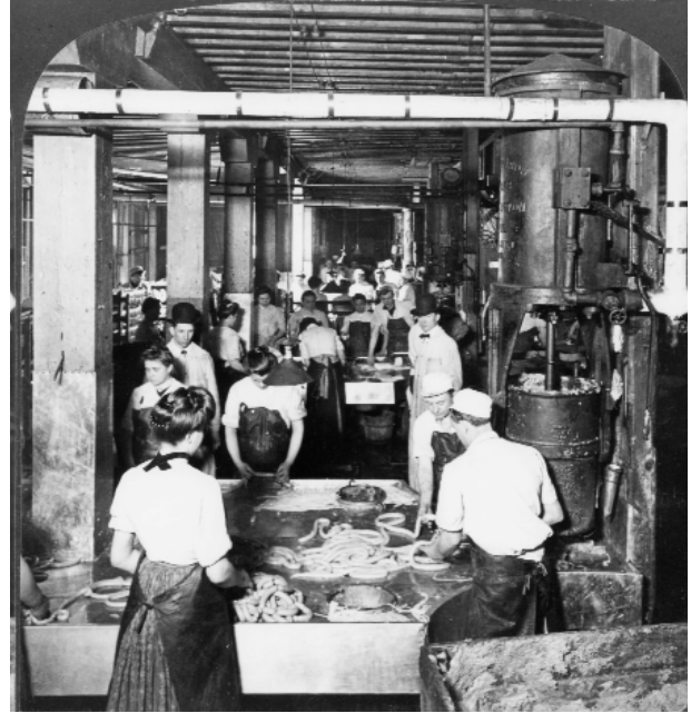
[7110] H. C. White Co., Making Link Sausages—Machines Stuff 10 Ft. per Second (c. 1905), courtesy of the Library of Congress [LC-USZ62-50217].
