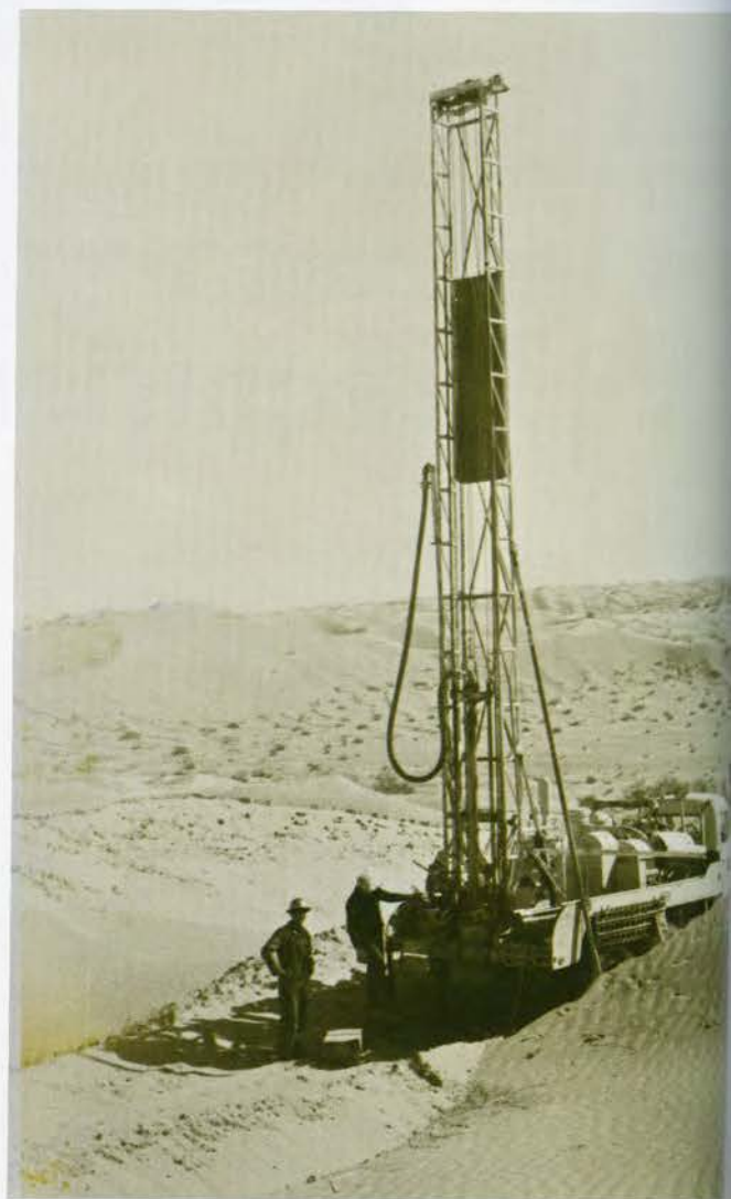
Below—Driller Giovanni Reale and his helper are drilling amongst hard-packed dunes after a bulldozer has cleared a spot for them.
