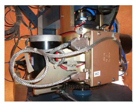
Figure 2: X/L band Polar Satellite Antenna Home Sensor
