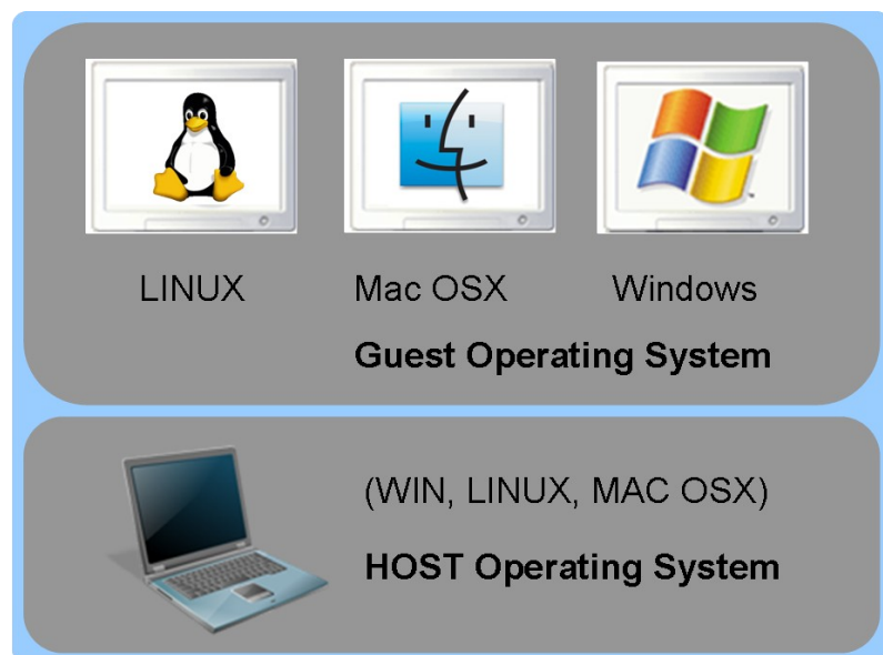
Figure 2: The virtual machine software installed on a host operating system allows the use of different operating systems on a single computer system. A Macintosh system could run native Windows or LINUX software or even multiple instances of the same operating system. All virtual machines can communicate with each other and are allowed to use all hardware computer resources such as graphic cards, DVD drives and USB ports. (Logo sources: Wikipedia, TUX mascot: Larry Ewing).
