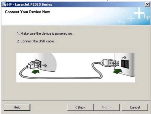
When the **Connect Your Device Now** screen appears, make sure that the HP LaserJet P2015 is turned on. Then attach the USB cable between the computer and the HP LaserJet P2015.
