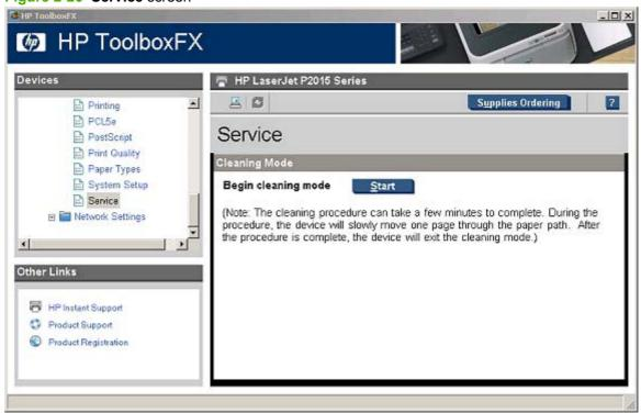
During the printing process, paper, toner, and dust particles accumulate inside the printer. Over time, this buildup can cause print-quality problems such as toner specks or smearing. Click **Start** to run the cleaning mode procedure on the HP LaserJet P2015 printer.
