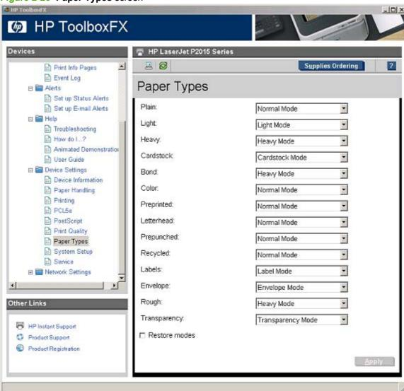
A print mode is a special setting that controls the print speed and the fuser temperature of the printer. The product speed and fuser temperature are adjusted to match the selected print mode, which can result in better print quality when printing on certain media types.
