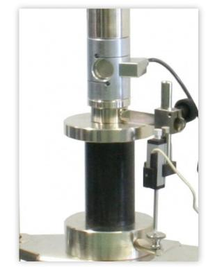
Figure 2. ASTM C39 Modulus Determination
