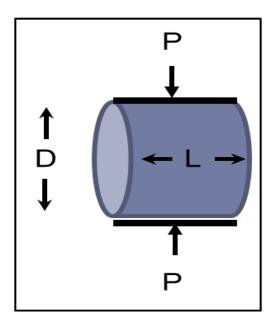
Figure 6 – Illustration of Splitting Test
