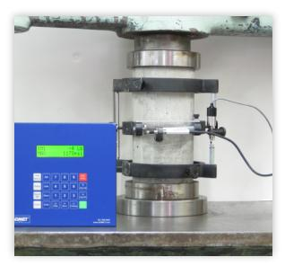
Figure 3. ASTM C469 Modulus Determination
