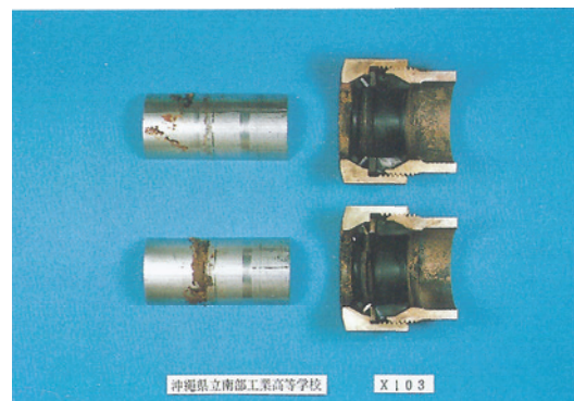
(6) Flexible (B) coupling (after pickling)
