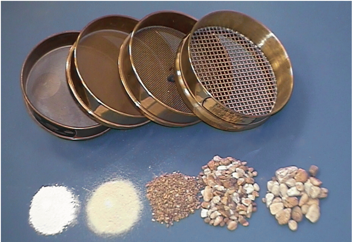
Figure 2-2. Example of laboratory sieves for mechanical analysis for grain size distributions. Shown (right to left) are sieve nos. 3/8-in (9.5-mm), No. 10 (2.0-mm), No. 40 (0.425 mm) and No. 200 (0.075 mm). Example soil particle sizes shown at the bottom of the photo include (right to left): medium gravel, fine gravel, medium-coarse sand, silt, and clay (kaolin) (FHWA, 2002b).
