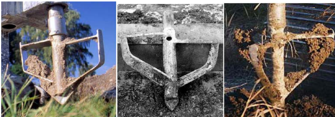
Figure 10: Nordic dry mixing "standard" tool (Larsson, 2005)
