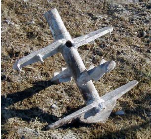
Figure 11: Nordic modified dry mixing tool (Larsson, 2005)
