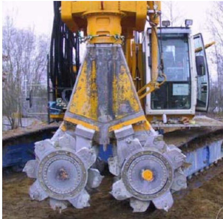
Figure 7: Bauer cutter soil mixing (Fiorotto et al, 2005)
